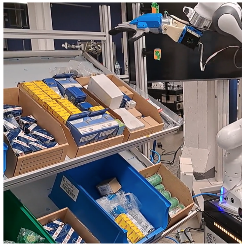
Figure 4: Dynamic manipulation with the general-purpose gripper
