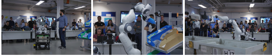
Figure 15: Impressions from the full scenario demonstration. DARKO robot approaching the shelf (left), a successful grasp of an item from a bin (middle), delivery and throw of the item into the target tray (right)
