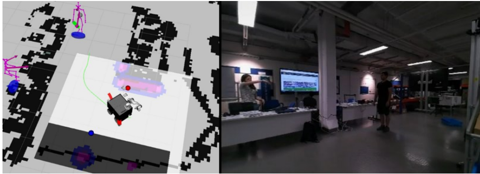
Figure 13: Focus on human skeletons detection and the constraints (blue and red markers) derived from the risk map.
