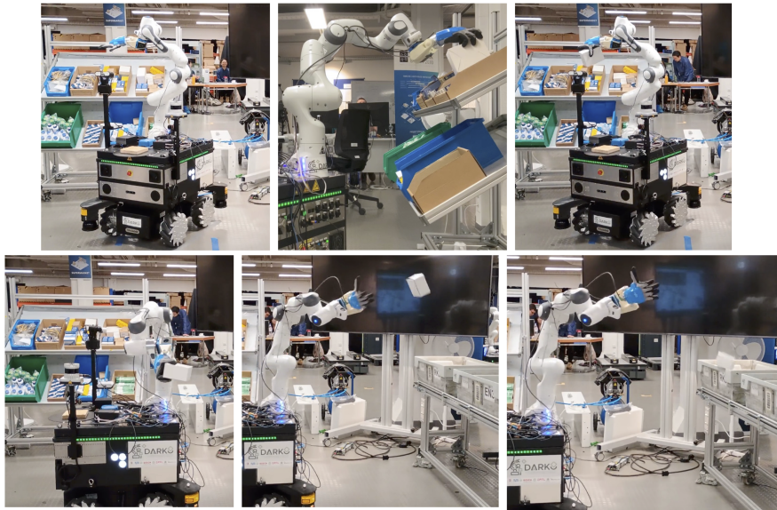
Figure 5: Single dynamic manipulation cycle of the use-case scenario
