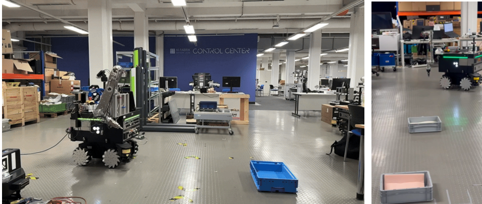
Figure 7: Throwing configuration during MS3 (left) and during MS4 (right). On the right picture, the box placed the closes to the robot corresponds to the throwing distance using only the rigid components of the BSA, while the second box indicates the longest throwing distance achieved by the elastic arm.
